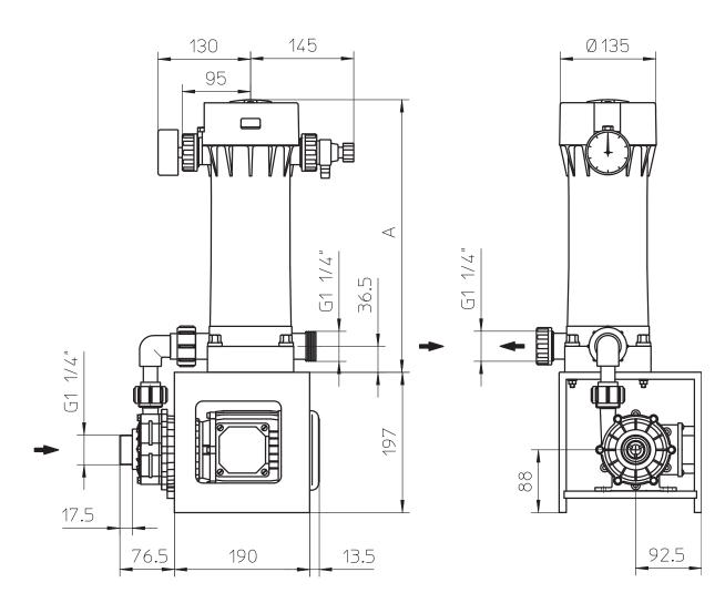
The dimensioned drawing shows a filter combined with a pump of type 1.5. Other combinations may have different dimensions.
